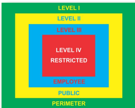
Figure 2: Physical security protection levels Source: Author
